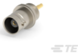
TE Part # 6-1337449-0 BNC BHSkt 50Ohm Nickel Pltd
