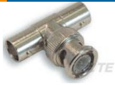
TE Part # 6-1337458-0 BNC T Adpt JPJ 50Ohm Nickel Gold Pltd
