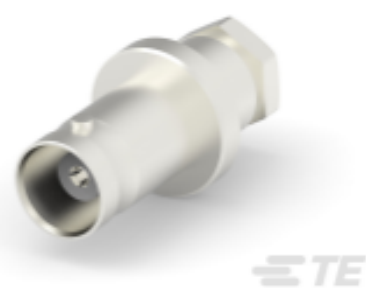
TE Part # 6-1478409-0 BNC Str Jk PS 50Ohm Silver Pltd RG58C/U,
